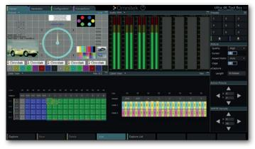
Instruments can be displayed as multi-tile (up to 9 on screen) or full screen.
